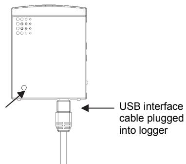
If the logger has never been connected to the computer before, it may take a few seconds for the new hardware to be detected. Use the logger software to launch and read out the logger.
