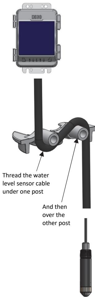
2. Insert the posts (with the cable routed as shown) into the receptacles in the other half, forming one disk when connected.
