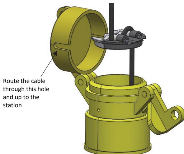
5. Close the well cap. Use a padlock to restrict access to the well if desired.
