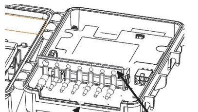
Notch where the key on the bottom of the cable channel is installed
