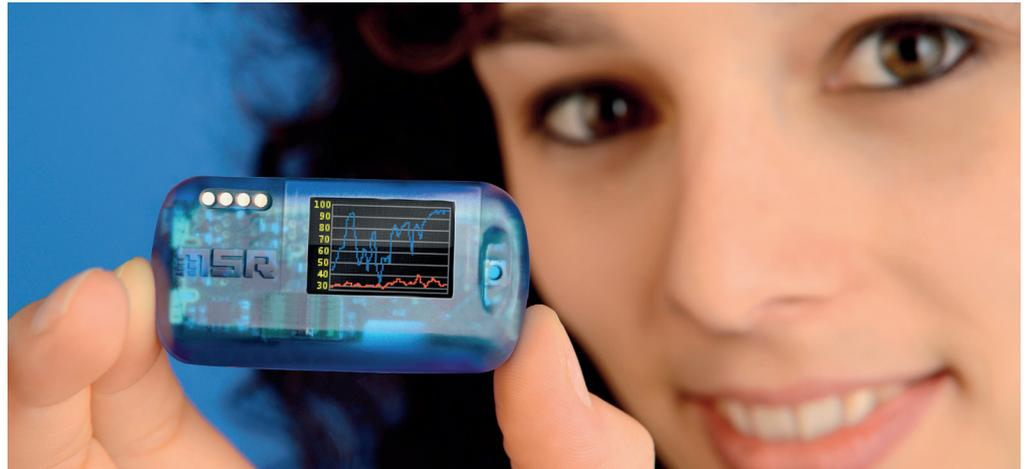
Wireless monitoring of measurement data and rapid reading of measured values – this ease of use is offered by the new MSR 145WD wireless data logger. The mini-logger is equipped with Bluetooth Low Energy, a bright OLED graphic display and the optional web-based service MSR SmartCloud for data monitoring from any location.
