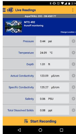
Use the VuSitu Mobile App to access and manage data on your Android™ smartphone or tablet. Intuitive, free mobile app is an all-in-one software package that provides auto-configuration, simplified calibration, guided log setup, directed data analysis, and automated report creation. Tag data with site photos and GPS coordinates. View results in the field and email data on the spot. Download through the Google Play Store.
