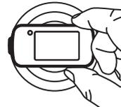
**8** To perform a daily logger check, connect to the logger (see step 5) and tap Perform Daily Check (A). To download the logger, connect to it and tap Download (B); choose Download and Stop if you want to restart the logger with a new configuration. Once downloaded, you can share the logger report immediately or access it later by tapping Reports (C).
