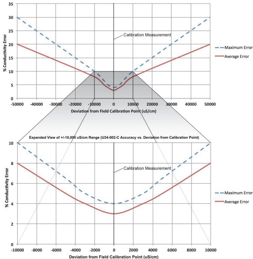
**Note:** The accuracy of the readings is relative to their proximity to the calibration point. The closer the conductivity reading is to the calibration point, the higher the accuracy. The calibration point is measured in actual conductivity (not specific conductance), while the calibrated data is provided in either specific conductance or salinity.
