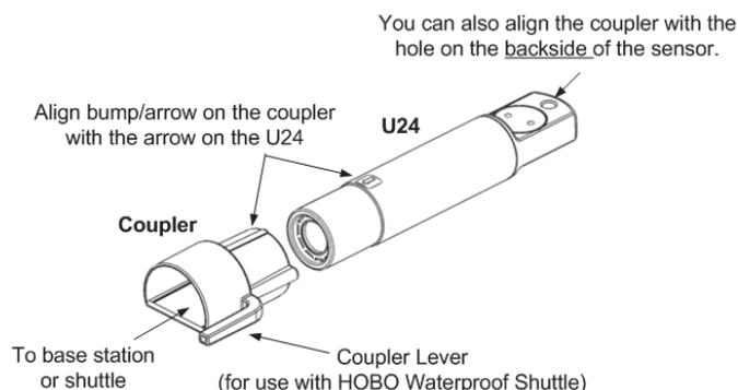
**WARNING:** Do not leave the logger in the coupler for extended periods of time. When connected to a coupler, the logger is “awake” and consumes significantly more power than when it is disconnected and considered “asleep.” Always remove the logger from the Optic Base Station or HOBO Waterproof Shuttle as soon as possible after launching, reading out, or checking the status to avoid draining the battery.
