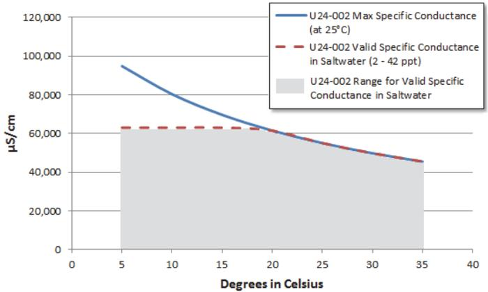
\* The Practical Salinity Scale 1978 (PSS-78) used to calculate salinity is valid for salinities in the range of 2 to 42 ppt. For salinities outside of this range, use the measured conductivity and temperature data from the logger with a calculation appropriate for your salinities.
