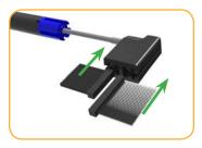
Insert the new small bristle set into the small slot. Slide the large bristle set into the large slot.
