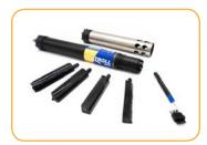
Uninstall all connected sensors and wiper or wiper port plug.
