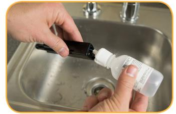
Insert the fill tube into the bottom of reservoir.
