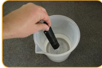
To remove crystalline deposits, clean with warm water and soap, or soak sensor in 5% HCl solution for 10 to 30 minutes.
