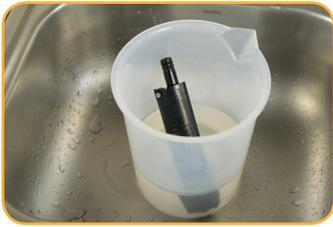
Soak sensor for a minimum of two hours in 140 mg/L ammonium as N standard or the highest standard you plan to use during calibration.
