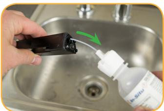
Squeeze a steady stream of solution into the reservoir while slowly pulling out the tube.
