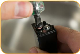
Remove sensor from sonde and unscrew reference junction.
