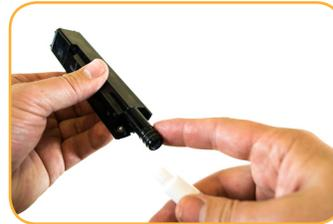
Lubricate o-ring at bottom of sensor.
