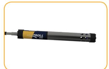
Flip the restrictor into deployment mode after calibration
