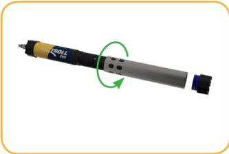
Remove restrictor from the instrument.
