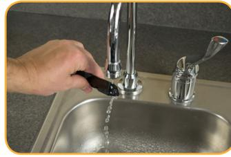
Soak overnight for the best long-term results. Rinse thoroughly with deionized water prior to calibration.
