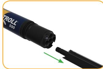
Remove sensor port plug if installed. Do not twist.
