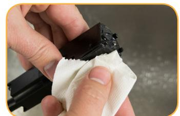
Wipe away excess solution. Soak in tap water for 15 minutes and calibrate.
