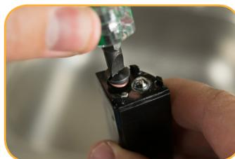
Overfill slightly. Reinstall reference junction cap and tighten until it touches sensor body.
