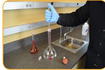
3. To obtain a 500 µg/L concentration, pipette 5 mL of the 100 mg/L solution into a 1000 mL flask.
