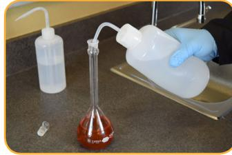
2. Bring the flask to volume with deionized water. The resulting solution is 100 mg/L Rhodamine WT.
