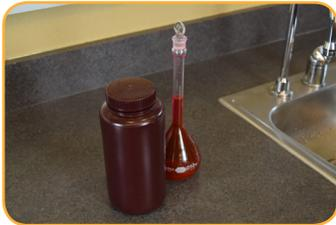
Use an opaque container to store the 100 mg/L solution in a cool, dark place for up to six months.
