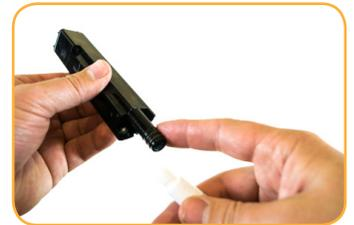
Lubricate o-ring at bottom of sensor.
