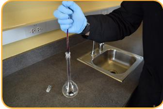
1. Start with a 2.5% Rhodamine WT solution. Pipette 1.0 mL of the solution into a 250 mL Class A volumetric flask.
