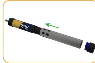
Place restrictor on instrument in calibration mode.
