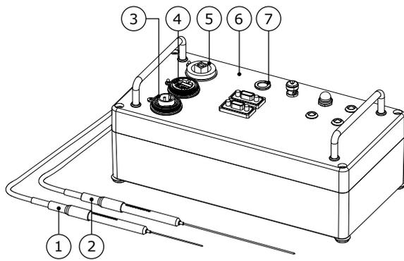
**Figure 5** overview of TPSYS20: the system includes needle model TP08 (1) or TP02 (2) and the MCU (6). The thermal needle probe must be connected to the MCU (7). The MCU is powered from a 12 VDC power source (3). Communication with the MCU can be done via Ethernet (4) or USB (5).
