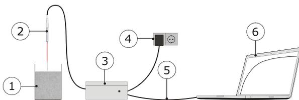
**Figure 3** TPSYS20 standard configuration: Sample (1), Needle model TP02 or TP08 (2), MCU Measurement and Control Unit (3), Adapter suitable for both 230 and 110 VAC (4), USB or ethernet connection (5), PC (not included) (6)
