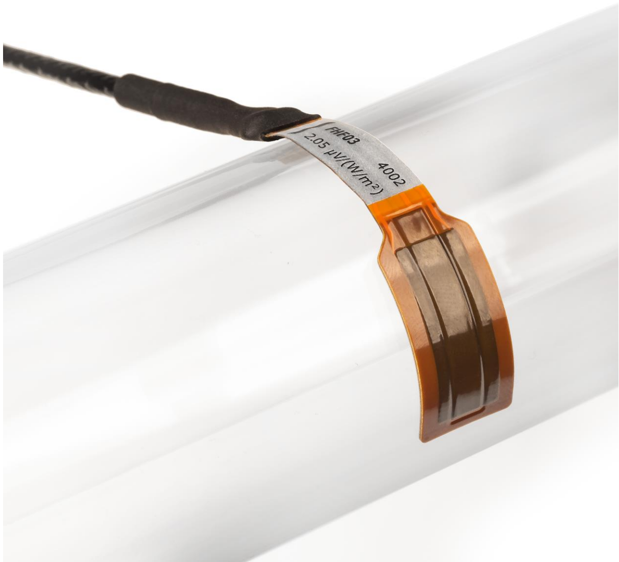
Figure 5.2.1 Bending of an FHF03 foil heat flux sensor, in this image on a pipe.
