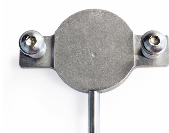
Figure 6 IHF01 with spring-loaded bolts for mounting on a well-prepared flat surface using tack-welded threads
