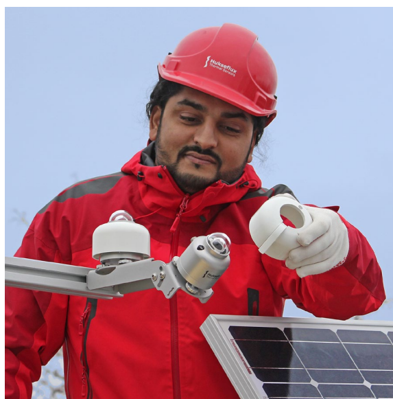
Figure 0.7 Hukseflux PMF series pyranometer mounting fixtures can be used for easy installation of pyranometers. On the left, PMF01 pyranometer mounting fixture with one SR30, and on the right PMF02 with two SR30 pyranometers. Both fixtures allow mounting in Plane of Array for PV system performance monitoring and meteorological applications.
