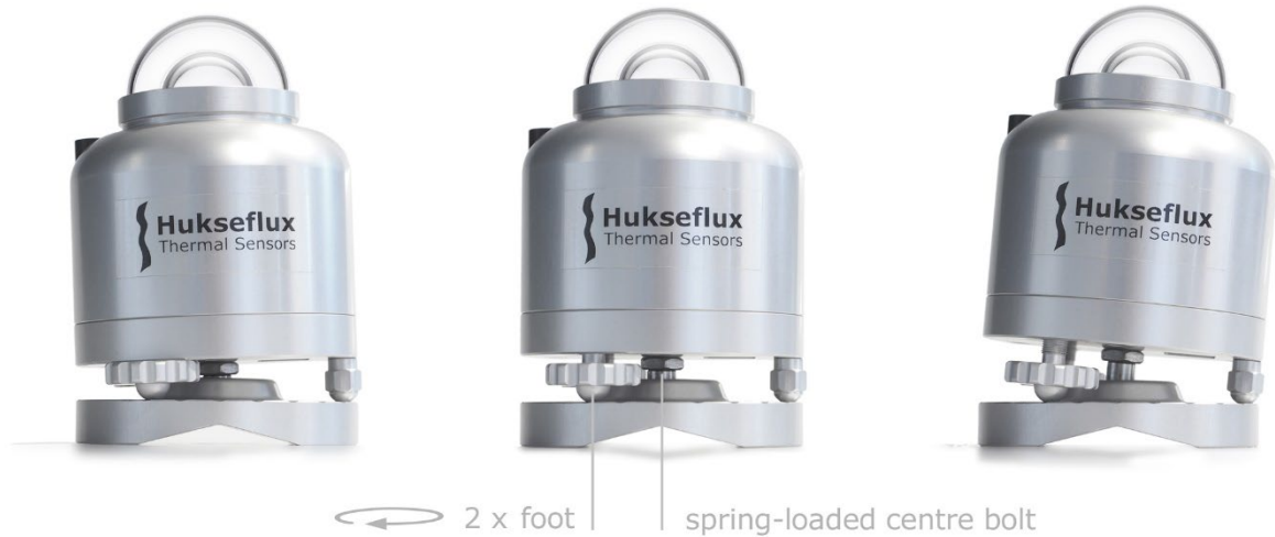
Figure 5.3.1.5 SR30 locked on its optional levelling mount: by fastening (on the left) or loosening (on the right) SR30's two adjustable feet, SR30 can be levelled, judging by the bubble level. SR30's static foot remains fixed. In all cases, ensure the legs of SR30 fit into one of the small ledges of the levelling mount. Locking is in place, when the nut is turned all the way against the bottom plate of SR30.
