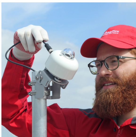
Figure 0.7 Hukseflux PMF series pyranometer mounting fixtures can be used for easy installation of pyranometers. On the left, PMF01 pyranometer mounting fixture with one SR30, and on the right PMF02 with two SR30 pyranometers. Both fixtures allow mounting in Plane of Array for PV system performance monitoring and meteorological applications.
