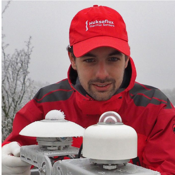
Figure 0.2 Heated to counter frost and dew deposition: clear difference between a non-heated pyranometer (back) and SR30 with RVH™ technology (front).
