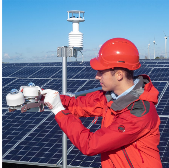
Figure 0.3 SR30 includes a digital tilt angle measurement, very practical for remote checks of instrument orientation. The image shows two SR30's in PV system monitoring, one measuring in Plane of Array (POA).
