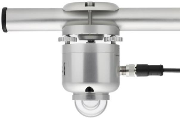
**Figure 3** the Tube mounts of SR30 and SR15 and SR05 can very well be used to measure global, reflected, and Plane Of Array irradiance. For downfacing instruments we typically do not use the sunscreen. See also Figure 1.
