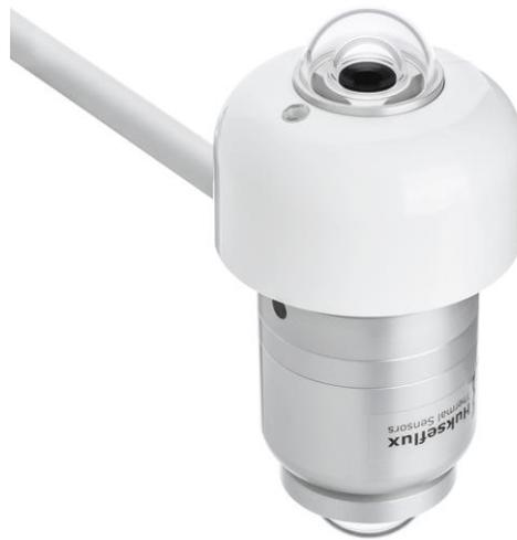
**Figure 2** 2 x S30 spectrally flat Class A (secondary standard) pyranometer connected to a fixture plus rod, together forming an albedometer. The downfacing pyranometer is equipped with a glare screen to block solar radiation entering the lower detector at low solar angles (150° instead of 180° full field of view angle).
