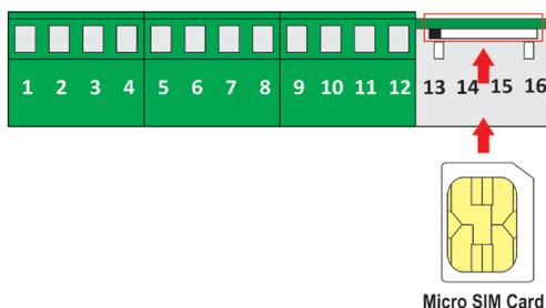
Fig. 39 – Conexão Micro SIM Card
